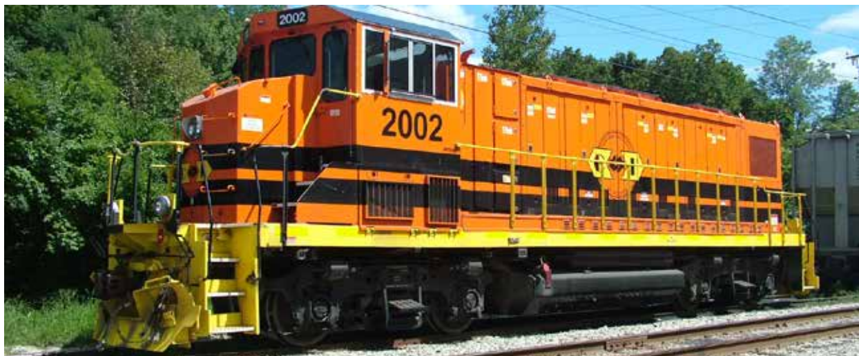
The DERG program provided funding to repower this switching locomotive, which operates near Cincinnati, OH. The locomotive's existing single diesel engine was replaced with three generator-set diesel engines, each of which runs only when its power is needed. Source: Ohio Rail Development Commission.
